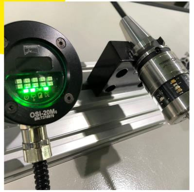
OPS-30 optical probe system include two pieces of hardware and one software package; The software package model is SP-W10, the two pieces of the hardware are: 1) OP510 optical probe (including optional shank and stylus); 2) OSI-20 optical receiver(the standard cable length 8m/the optional lengthened cable).
